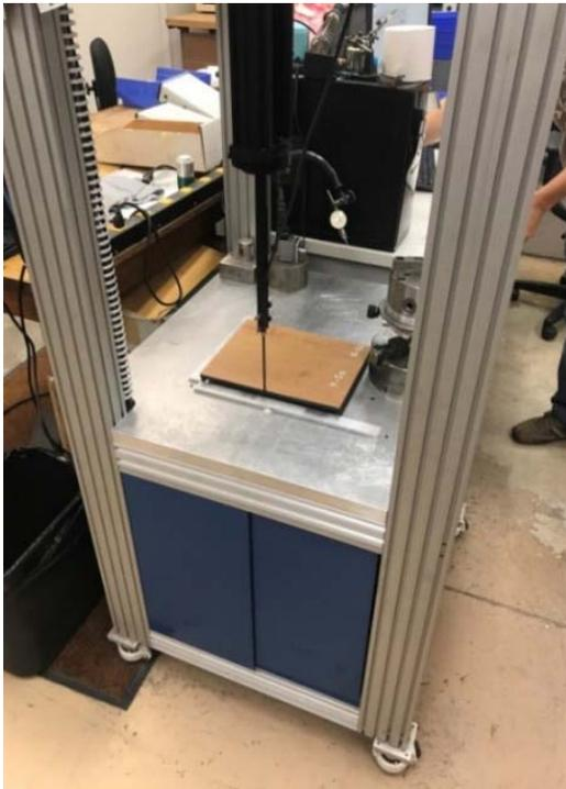
Fig. 7. Photograph of the magnetic field test on the surface of magnetic floors (D1-A and D1-B) with the presence of the magnetic subfloor.
