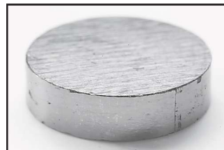
Photo 1: This is a sample of Niron Magnetics’ novel iron nitride-based Clean Earth Magnet (Image Source: Niron Magnetics)
